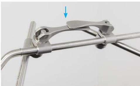
**✓** Before locking, rotate crossbar cam joint handles out of the way so that they do not block the crossbar.
